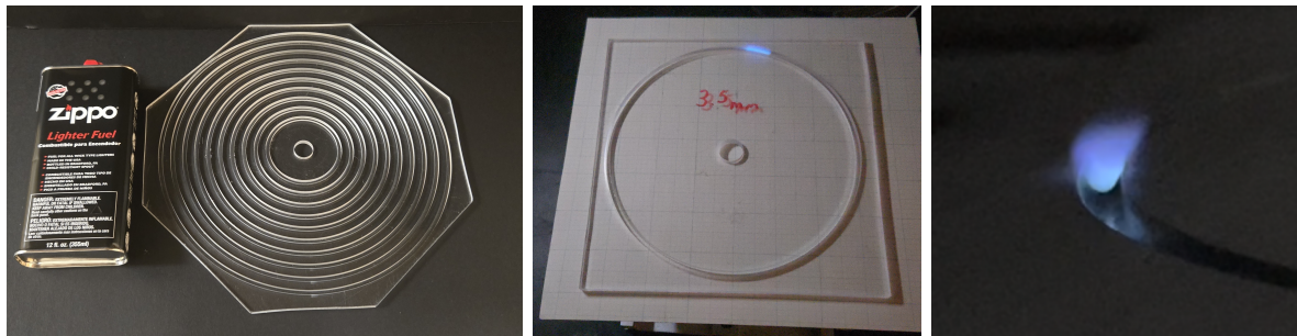
Figure 2: Left: Zippo Lighter Fluid bottle and acrylic mold containing eight channels. The annular radii vary from R = 30 mm to R = 120 mm. Center: Blue flame pulse propagating in an acrylic annular channel. Right: Close-up of a propagating flame pulse in an aluminum annular channel. Hovering of the pulse above the fluid is clearly visible.
