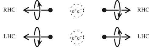
Figure 1.18: Positronium (top) annihilates into a pair of right circular photons (middle) or a pair of left circular photons (bottom). Both possibilities superpose to form an entangled state. The photon emission is isotropic.
