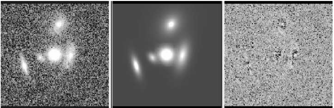
FIG. 2: An example GALFIT output file. The original image is on the left, the modeled objects are in the middle, and the residual background light is on the right.
