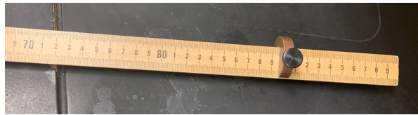
FIG. 3: Our physical pendulum, composed of a meter stick with a (60.0 \pm 0.1) g sliding mass attached at (90.0 \pm 0.1) cm.
