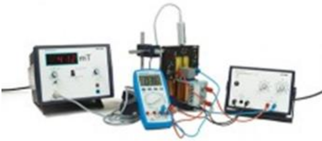
FIG. 2: The experimental apparatus for the experiment. From the left is the gauss meter, the volt meter, the Hall effect module, with a board inserted, the magnetic coils, and the power source for the coils. Credit to PHYWE [3]
