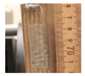
FIG. 8: One of the images for the shaved ball being analyzed. Each image was analyzed using this method to record the distance the spring stretched. The red lines were used to more accurately determine the distance the spring was stretched.
