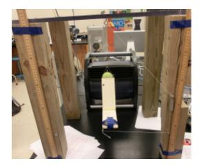
FIG. 3: An image of the entire apparatus. The board is hung by a string from a plexiglas table top in front of the fan. As the board rotated, the horizontal string would be pulled, stretching the spring to a certain equilibrium distance that could be recorded using the meter stick.
