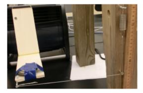
FIG. 5: A close up of the region where the board was attached to the spring. As the board rotates clockwise due to the Magnus force, the string is pulled horizontally by the back of the board. The string then is routed around the nail and pulls downward on the spring. The distance the spring stretched will vary until the two forces each equilibrium, and then the distance can be recorded using the meter stick.
