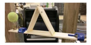
FIG. 2: An image of the main section of the apparatus. On the left is the tennis ball which is mounted on the high rpm motor. Just right of that is the battery which is taped to the board with blue duct tape. The two boards in the middle form a triangle to hang the board by and keep it from bowing due to the weight at either end. On the far right are the counter weights which are attached to the board using blue duct tape.
