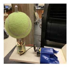
FIG. 4: An image of the tennis ball skewered by the aluminum rod. The skewer is attached to the motor with the black set screw. The battery has been attached to the board with duct tape and the motor is sitting in a small hole in the board and attached to it using hot glue.
