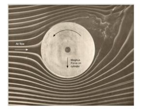
FIG. 1: An image of a cylinder in a wind tunnel with fog tracers. The cylinder is rotating counter-clockwise as seen by the arrow. The airflow is coming from the left which can also seen by an arrow. This creates a Magnus force on the cylinder that acts downward. [4]
