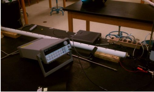
FIG. 1: An view of the acoustic metamaterial with microphone, speaker, and waveform generator.
