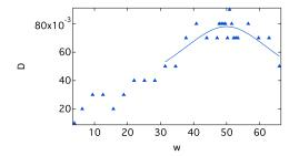
FIG. 5: Amplitude of Oscillation (meters) vs  $\omega$  (Hz). Q value is  $\omega_0$ /FWHM where  $\omega_0$  is the resonance frequency. This is for the bridge deck made of birch wood.
