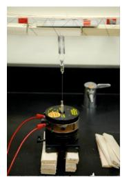
FIG. 3: PASCO driver attached to the side of the bridge deck.
