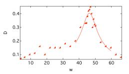
FIG. 6: Amplitude of Oscillation (meters) vs  $\omega$  (Hz). Q value is  $\omega_0$ /FWHM where  $\omega_0$  is the resonance frequency. This is for the bridge deck made of balsa wood with holes drilled into it.
