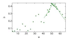
FIG. 4: Amplitude of Oscillation (meters) vs  $\omega$  (Hz). Q value is  $\omega_0$ /FWHM where  $\omega_0$  is the resonance frequency. This is for the bridge deck made of balsa wood.
