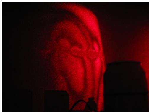
Figure 3: I was able to count three fringes using the pictured hologram. The ovals are not easily discernable as they merge in several areas. But if you look at the central band on the cans projection three general ovals can be found.
