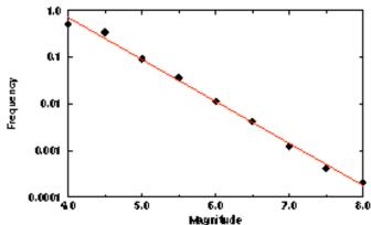
Figure 1: An example of the Gutenberg-Richter law. The data was taken from earthquakes that occurred around the world in 1995 From Reference [4].
