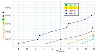
Figure 4: An example of the data obtained from Data Studio, using photogates to monitor the movement of each block, with each line representing a different block.
