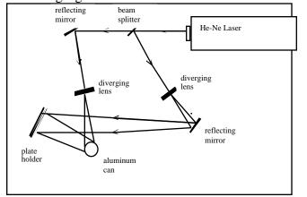
**Figure 1:** The beam from the laser is split into two beams, each directed through a diverging lens. Light waves from one lens fall on the object and are reflected onto the plate holder. Light waves from the other lens are reflected onto the plate holder by a reflecting mirror.
