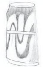
**Figure 2:** Interference fringes can be seen on an aluminum can when a double exposure hologram is made. The first exposure is taken with a rubber band around the center of the can, while the second exposure is taken once the rubber band is removed.
