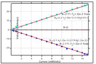
Graph 2: Current plotted against voltage, corrected for systematic error, such that there is no voltage reading for B=0. Straight lines are fitted to the data. The markers are consistent with graph 1.
