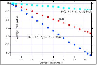
Graph 1: Transverse (Hall) Voltage plotted against the longitudinal current, uncorrected for systematic errors. The opaque squares and circles are voltages for opposite orientations of the magnetic field, while the crosses are voltages in the presence of no magnetic field.
