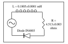
Figure. 1. Circuit diagram of setup for a driven nonlinear electrical oscillator. A function generator creates a current that travels through a conductor, resistor, and a diode.
