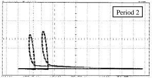
Figure 2. Phase space diagram of  $V_0$  versus  $V_s$  at Frequency = 180.0 KHz and Amplitude = 2.985  $V_{pp}$ . Period 2 is seen here as two peaks.
