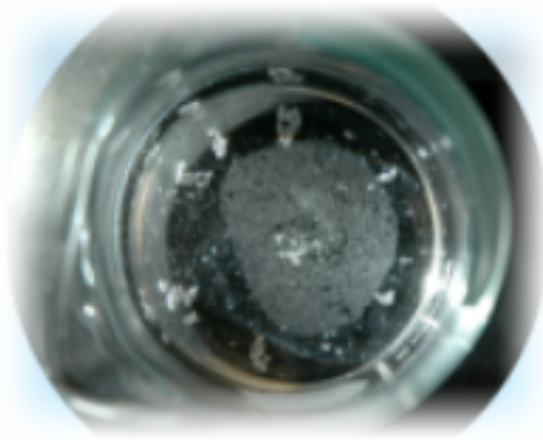
Upon heating and freezing, the hard water solutes precipitated out of the water. Precipitates both sank (large clusters) and floated (blurry circle).
