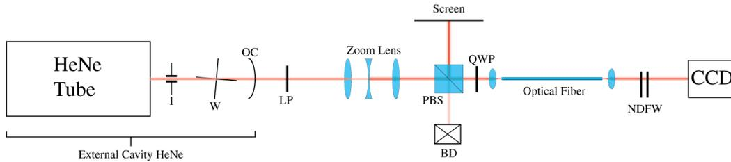
**Fig. 1** Experimental setup. OC = output coupler. W = crossed wires. LP = linear polarizer. PBS = polarizing beam splitter. QWP = quarter-wave plate. NDFW = neutral density filter wheel. BD = beam dump. CCD = charge-coupled device camera. The linear polarizer is set to horizontal polarization. The QWP is set to create left- or right-circularly polarized light.
