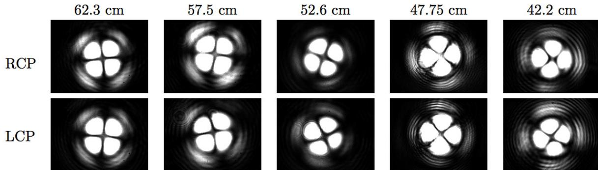
**Fig. 2** Images of a subset of the recorded output modes illustrating the rotation. The fiber length traversed is indicated across the top and the input circular polarization is denoted on the left.
