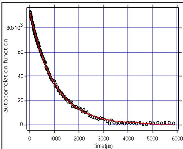
FIG. 3. Graph of the autocorrelation function (arbitrary units) versus time ( $\mu\text{s}$ ) for Run 1 of the polystyrene mixture. The dots represent the experimental data while the solid line is the theoretical fit.
