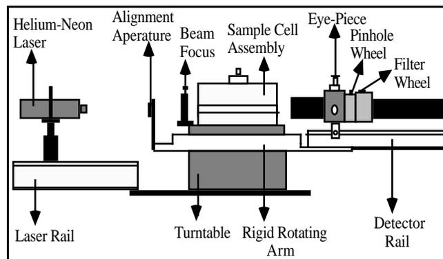
FIG. 2. Diagram of the BI-200 SM Goniometer with the major features labeled.
