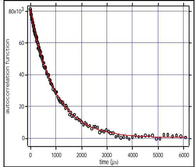
FIG. 4. Graph of the autocorrelation function (arbitrary units) versus time ( $\mu\text{s}$ ) for Run 2 of the polystyrene mixture. The dots represent the experimental data while the solid line is the theoretical fit.
