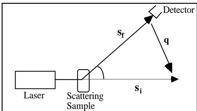
FIG. 1. The incident wave vector,  $s_i$ , is scattered in all directions upon reaching the scattering sample, but only the light of the wave vector  $s_f$  is detected. The geometry of the apparatus defines the scattering vector  $q$  where the angle is called the scattering angle.
