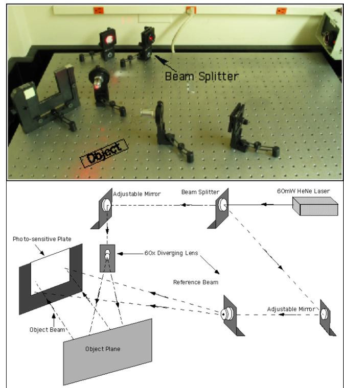
Figure 1: Diagram and photograph of the transmission hologram optical setup in The College of Wooster darkroom. Shiny surfaces, such as the optics bench and the light colored wall were covered with black cloth to cut down on fogging of the film plate during exposure.
