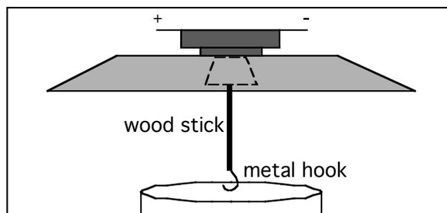
Figure 2: Modified speaker with a wooden probe cemented in the center cone. The metal hook touches the center of the can's top.
