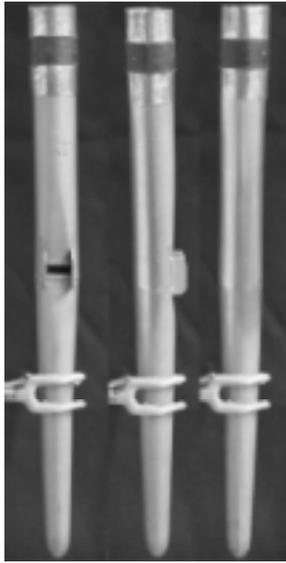
Figure 4: G4 principal diapason organ pipe, front, side and rear view. Notice the shiny surface on the rear of the pipe, a result of polishing the surface with crocus cloth.
