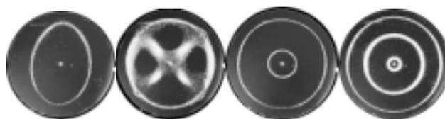
Figure 3: Chladni plate modes using sand to illustrate the node lines. These images were captured with a digital camera. The modes are, (left to right), [0,1] [2,1] [0,2] [0,3]. The actual frequencies of these modes are 107Hz, 360Hz, 460Hz 863Hz, respectively. These frequencies are accurate to within +/- 2 Hz.
