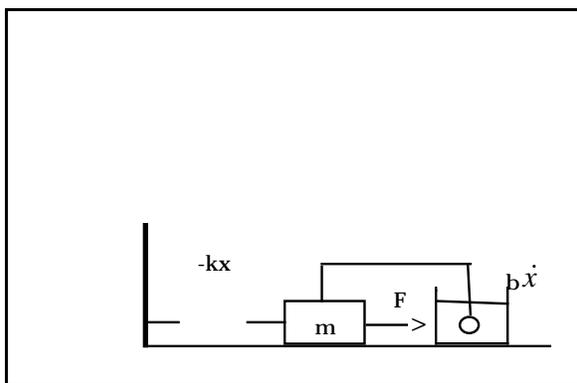
Figure 1: A simplified diagram of a damped harmonic oscillator.
