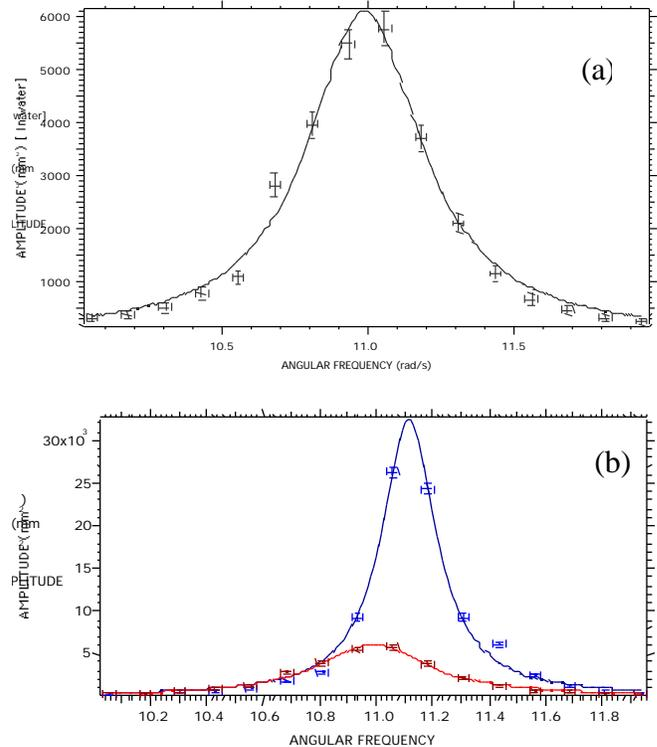
Figure 2: Amplitude squared versus angular frequency for (a) water, and (b) water and air compared. Note the shift in the resonant frequency.
