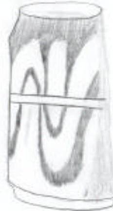
**Figure 2:** Interference fringes can be seen on an aluminum can when a double exposure hologram is made. The first exposure is taken with a rubber band around the center of the can, while the second exposure is taken once the rubber band is removed.
