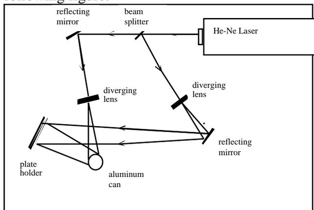
**Figure 1:** The beam from the laser is split into two beams, each directed through a diverging lens. Light waves from one lens fall on the object and are reflected onto the plate holder. Light waves from the other lens are reflected onto the plate holder by a reflecting mirror.
