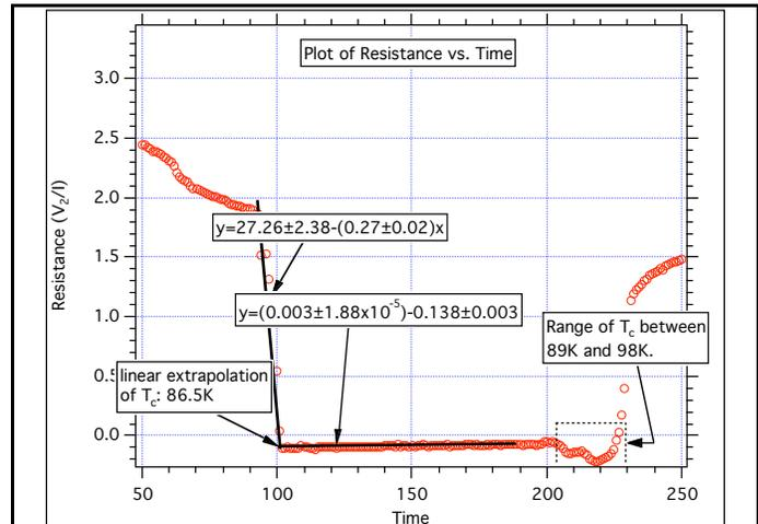
Figure 2, shows the plot of SC resistance versus time. Using a linear extrapolation, the analysis of the collected data yielded a result of  $T_c = 86 \pm 13\text{K}$  for the SC cooling, and a determined range between 89 and 98K ( $94 \pm 4\text{K}$ ) when heating the SC. The cooling process is the left side, and the heating process is to the right side.
