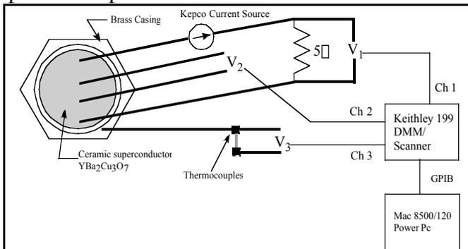
Figure 1 shows the complete set-up as was used in this experiment. Here  $V_1$  measures the current through the circuit,  $V_2$  measures the resistance across the ceramic SC, and  $V_3$  measures the temperatures via a thermocouple.
