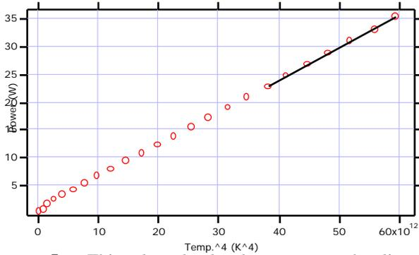
**Figure 5.** This plot clearly demonstrates the linear relationship between P and  $T^4$  at higher temperatures.
