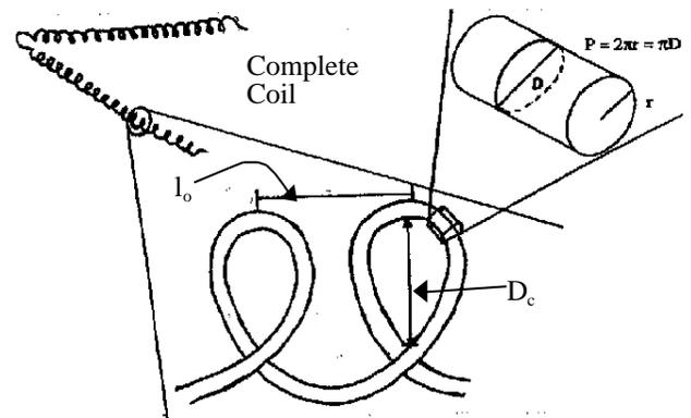
Figure 2. Schematic of filament
