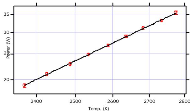
Figure 4. At high temperatures this log-log plot represents a straight of slope 4, which is the power of  $T$ .
