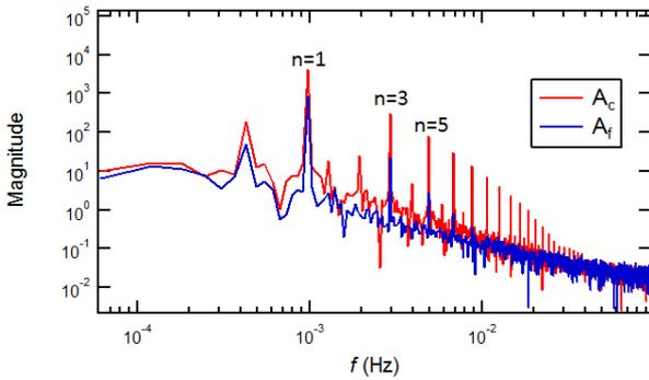
FIG. 4: The amplitudes of both Fourier transforms, graphed together. Manifesting peaks at the same frequencies, the blue  $\gamma_f$  peaks, further from the heat source, diminish much more quickly than the closer red  $\gamma_c$ , due to the dispersion of heat within the rod and emission of heat into the air. The peaks for the first, third, and fifth harmonics are shown, at 0.00098 Hz, 0.0029 Hz, and 0.0049 Hz, respectively.
