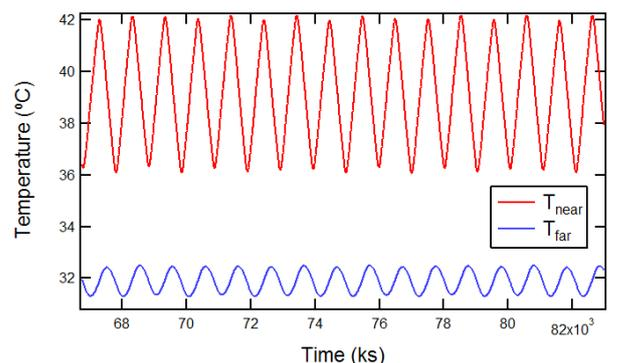
FIG. 3: A closer look at the region of data over which the Fourier Analysis was applied. The temperature close to the heated end is in red and the far temperature is in blue. There is an uncertainty of  $\pm 0.1$  C in  $T_c$  and an uncertainty of  $\pm 0.05$  C in  $T_f$ .
