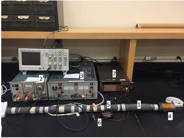
FIG. 1: Ångström experiment equipment. 1: Foam-wrapped brass rod. 2: Tektronix FG 501 function generator. 3: Kepco BOP 100 Power Supply. 4: Heater reservoir. 5: Two YSI 44004 Precision thermistors (embedded in rod). 6: 1.5 V dry cell battery and switch. 7: Keithley 199 scanner.
