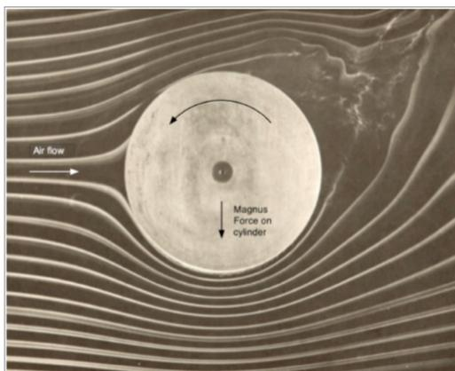
FIG. 1: An image of a cylinder in a wind tunnel with fog tracers. The cylinder is rotating counter-clockwise as seen by the arrow. The airflow is coming from the left which can also be seen by an arrow. This creates a Magnus force on the cylinder that acts downward. [4]
