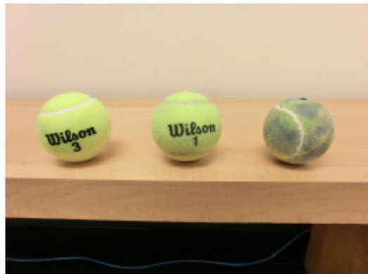
FIG. 6: The three balls used in the experiment. Starting from the left, the new ball, the shaved ball, and the furless ball.
