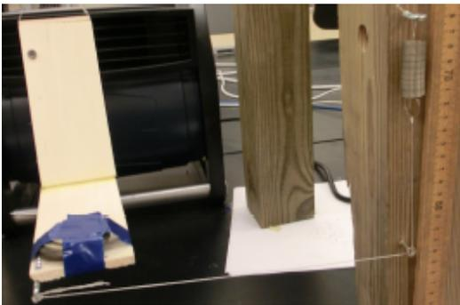
FIG. 5: A close up of the region where the board was attached to the spring. As the board rotates clockwise due to the Magnus force, the string is pulled horizontally by the back of the board. The string is then routed around the nail and pulls downward on the spring. The distance the spring stretched will vary until the two forces reach equilibrium, and then the distance can be recorded using the meter stick.
