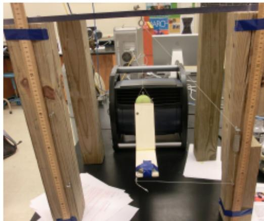
FIG. 3: An image of the entire apparatus. The board is hung by a string from a plexiglas table top in front of the fan. As the board rotated, the horizontal string would be pulled, stretching the spring to a certain equilibrium distance that could be recorded using the meter stick.
