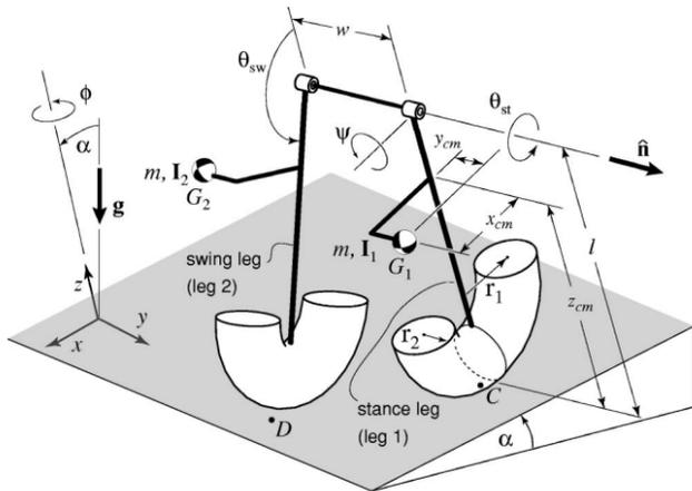
FIG. 2. Theoretical setup of a passive walker. This diagram is from the Cornell group’s paper “Prediction of stable walking for a toy that cannot stand” and it connects the dimensions discussed in the Cornell group’s theory and computational papers to their physical toy model [1]. This group eventually discovered that their simple simulations did not accurately predict the behavior of their passive robot.
