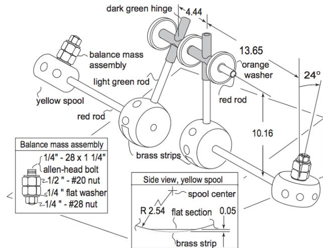
FIG. 3. Diagram of the Tinkertoy passive walking robot created by the Cornell group. This picture specifies the measurements of each part necessary to create a stable passive walking robot. We used this as a start-off point to create our initial robot. [2]. The overall mass of their walker was approximately 120 g with average foot balances of 50 g.
