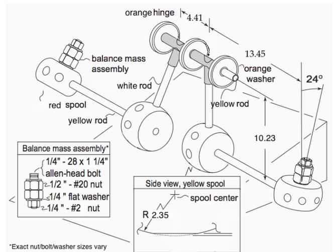
FIG. 4. Diagram of the Tinkertoy passive walking robot created by the Wooster group. This picture specifies the measurements of each part of our passive walking robot. We used the Cornell group’s diagram as a base for our own and only a measurements varied [2]. The overall mass of our walker was  $145.79 \pm 0.03$  g with the average of the masses on the foot balances being  $41.08 \pm 0.02$  g.
