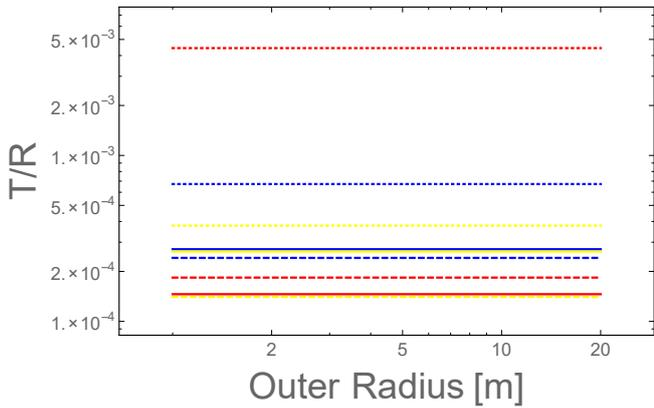
FIG. 4: A logarithmic plot of thickness divided by outer radius as a function of outer radius for aluminum (red), carbon fiber composite (blue), and graphene (yellow). The buoyancy conditions, stress conditions, and buckling conditions for each material are represented by solid, dashed, and dotted lines respectively.
