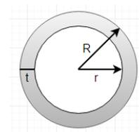
FIG. 1: Cross section of a vacuum lift cell with inner radius  $r$ , outer radius  $R$ , and thickness  $t$ .
