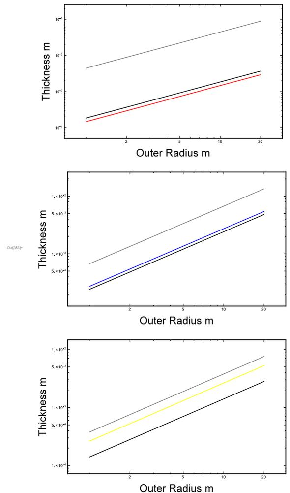
FIG. 3: logarithmic plots of thickness as a function of radius for the neutral buoyancy of aluminum 6061-T6 (red), standard modulus carbon fiber composite (blue), and multi-layer graphene (yellow). The neutral buoyancy condition for each material is plotted with its respective critical stress (black) and critical buckling pressure (gray).
