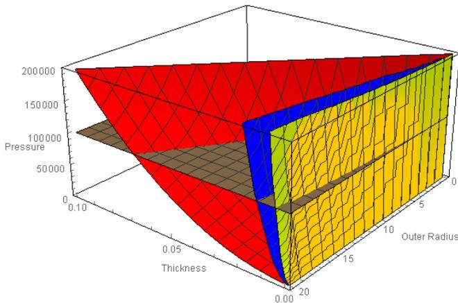
FIG. 2: A plot of the critical buckling curves for aluminum 6061-T6 (red), standard modulus carbon fiber composite (blue), and graphene (yellow). Atmospheric pressure at sea level is represented in gray. All points above this plane show combinations of thickness and radius that would be able to resist Earth's atmospheric pressure at sea level, while points below the plane show combinations that would fail to do so.
