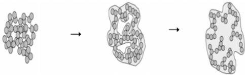
FIG. 1: Example of expansion. In the first panel the Osorb<sup>®</sup> is in its shrunken state. When the solvent is introduced in the second panel the Osorb<sup>®</sup> begins to adsorb the solvent. In the last panel The cross-linking structure is being broken down to allow for the absorption of the solvent by the Osorb<sup>®</sup>. [4]
