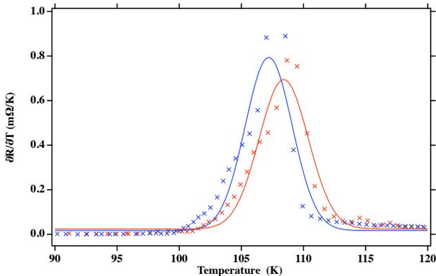
FIG. 4: Graph describing the derivative of resistance as a function of temperature,  $\partial R/\partial T$  vs  $T$  along with a Gaussian fit. The red data were taken using a current of 200 mA, while the blue data were collected using a current of 400 mA.
