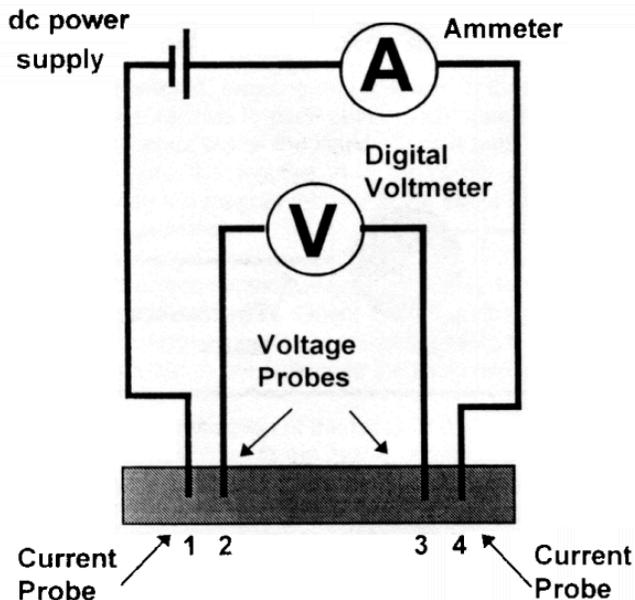
FIG. 2: Circuit diagram of the four-point probe. A digital multimeter was used to measure the current and the voltage.
