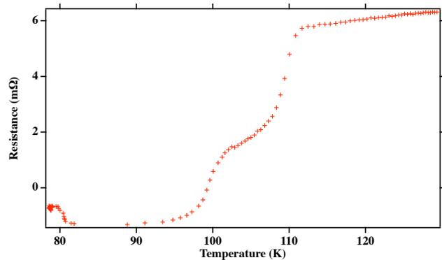
FIG. 5: Graph showing the unusual behavior of the resistance as a function of temperature at low current. For this run the current had a value of 10 mA.
