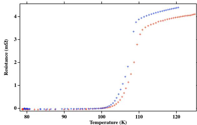
FIG. 3: Graph describing the resistance as a function of temperature. The red data were taken using a current of 200 mA, while the blue data were collected using a current of 400 mA.
