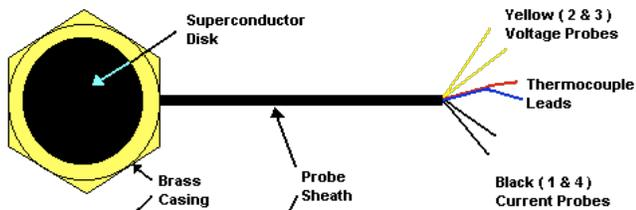
FIG. 1: Schematic representation of the four-point probe along with the YBCO superconductor in the brass casing.
