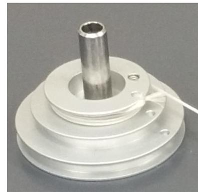
FIG. 2: A close view of the step pulley.
