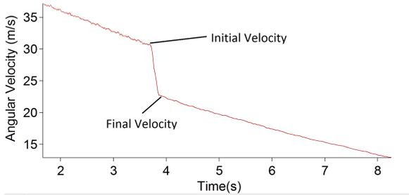
FIG. 6: This is the plot used to find the velocity before and after the ring was added to the apparatus.
