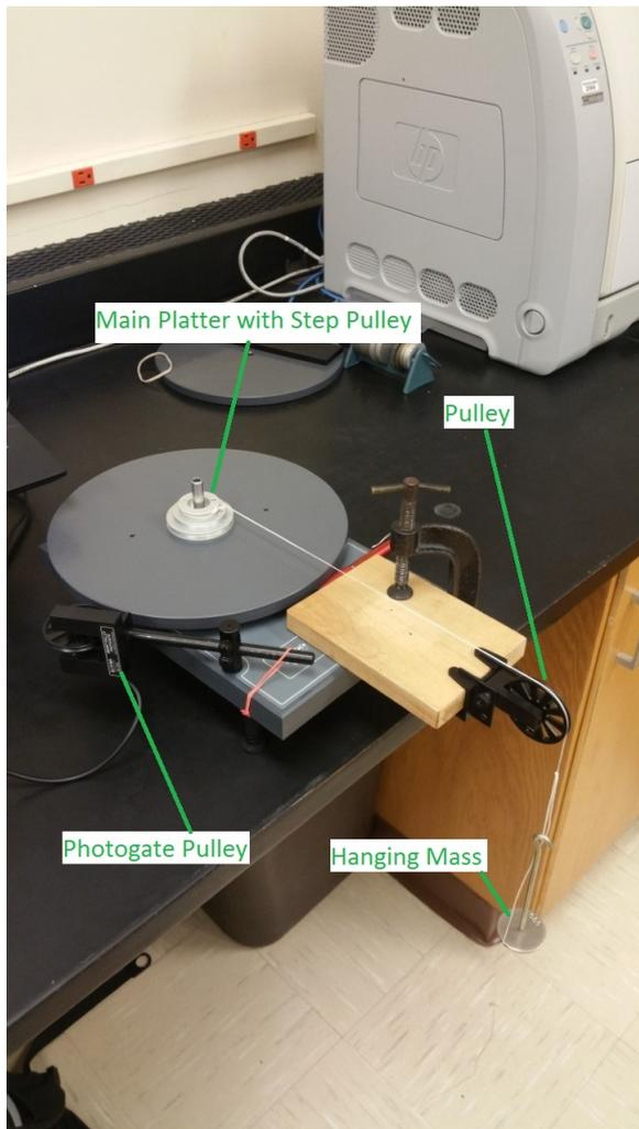
FIG. 1: The general apparatus used for the two experiments.
