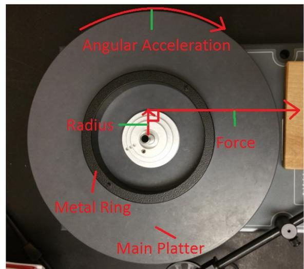
FIG. 3: The rotational apparatus with the ring, which was used to check for the conservation of angular momentum.
