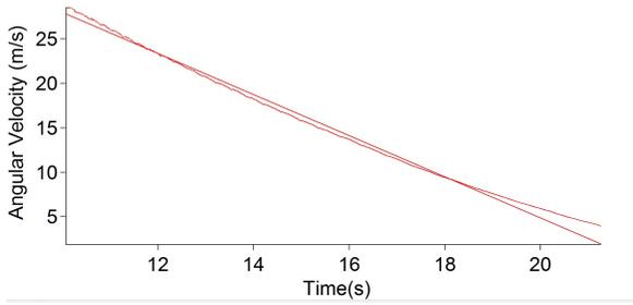
FIG. 5: This graph shows the velocity measurements that were used to calculate the friction of the apparatus.
