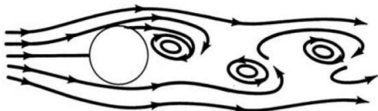
FIG. 1: Vortices alternately shedding off of a circular object in a fluid flow. This figure is reproduced from reference [3].
