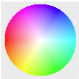
FIG. 3: The color coded velocity legend. The colors describe the direction of the velocity of the fluid while the saturation describes the magnitude. For example, the aqua blue color is fluid moving to the right and the red is fluid moving backwards, with the darker red fluid moving at a greater velocity than the paler red.
