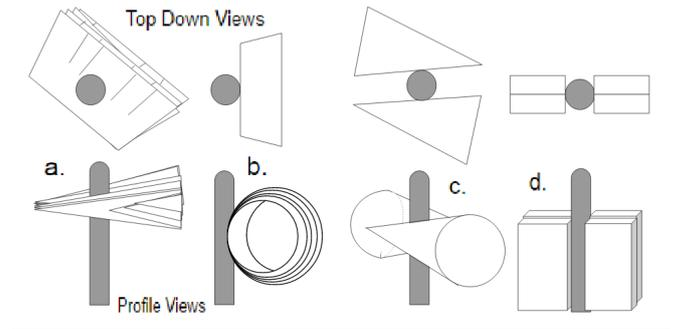
FIG. 1: The Top down and profile schematics for each flag a. TailFeatherFlag b. OnionSliceFlag c. DoubleWindsockFlag d. MassiveFlag
