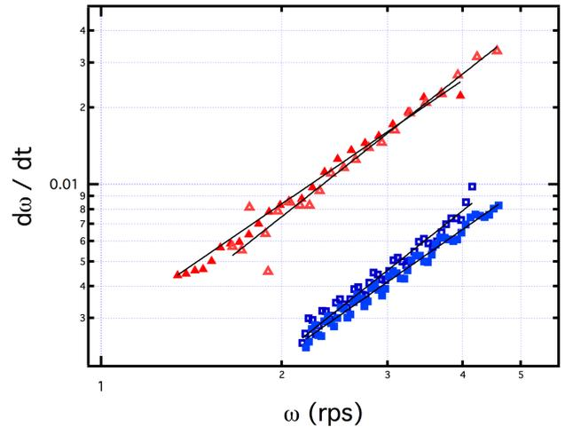
FIG. 4: Angular Acceleration  $d\omega/dt$  versus  $\omega$  for the Onion-SliceFlag and DoubleWindSockFlag. The solid identifiers correspond to counter clockwise rotation as specified in Table I.
