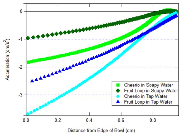
FIG. 11: The graphs of the differentiated accelerations versus the polynomial fit line of the data runs in Fig. 10. From top to bottom: a fruit loop in soapy water, a cheerio in soapy water, a fruit loop in tap water and a cheerio in tap water.
