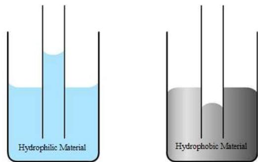
FIG. 1: The meniscus created between a hydrophilic material and water creates a positive meniscus as seen on the left. Between a hydrophobic material and water the meniscus created is negative, as seen on the right. In a hydrophilic capillary tube the meniscus raises the water level above the level outside the tube. A hydrophobic capillary tube would push the level of water in the tube below the outside level. Image from reference [5].
