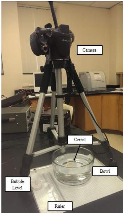
FIG. 4: A Casio High-speed camera was placed above the bowl so that the video was taken from directly above the bowl. The bowl was placed on graph paper so that the deformation of the surface of the water could be seen from above, as it distorted the image of the gridlines.
