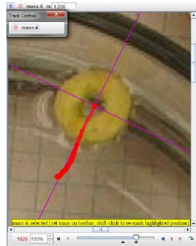
FIG. 8: An example of a video track for a fruit loop in water. The red trail is the motion of the center of mass over the selected frame range. The purple lines are the coordinate axes. The origin is set to the center of the cereal when it is at rest against the wall of the bowl to normalize the tracks for different size cereals.
