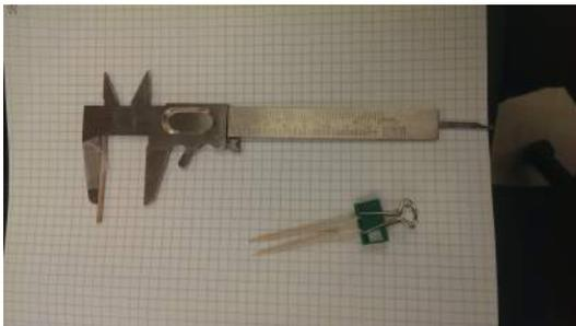
FIG. 5: A set of calipers were modified with a toothpick so that the toothpick could be placed in the open center of the cheerio. This insured that the cereal started at rest before drifting toward the side of the bowl. The clip with toothpicks attached, next to the calipers in the figure, held the cereal on the modified calipers until the calipers were in place to hold the cereal at the desired distance from the edge of the bowl.
