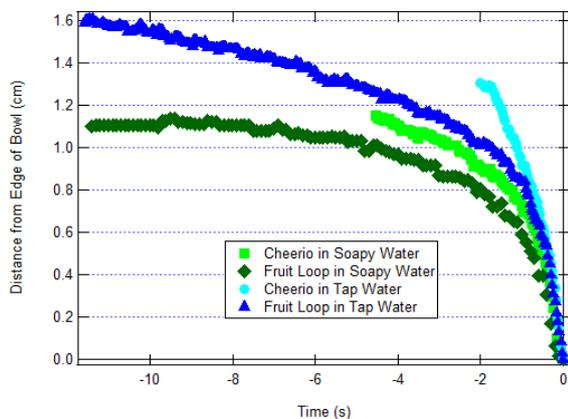
FIG. 10: The plot of position versus time for two different sizes of cereal in two liquids with different surface tensions. From left to right: a fruit loop in soapy water, a cheerio in soapy water, a fruit loop in tap water and a cheerio in tap water.
