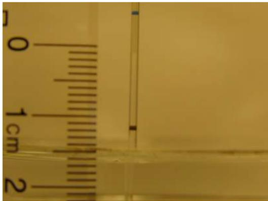
FIG. 7: Picture of the rise of the liquid in a capillary tube from the side. The distance between stripes on the tube was measured to be  $1.769 \pm 0.03$  cm. This value was used to calibrate Tracker to measure the rise in the capillary tube in the picture.
