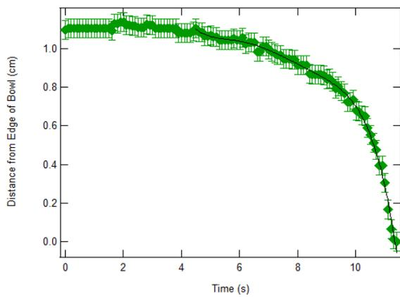
FIG. 9: The graph of position versus time for a fruit loop in soapy water. The data are shown as green diamonds, the sixth order polynomial fit line is shown in black.
