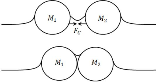
FIG. 2: The menisci surrounding two nearby particles combine to form a single meniscus between the particles, pulling them close together until the body of the particle prevents the meniscus from shortening further.
