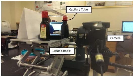
FIG. 6: Set up of camera, capillary tube, and liquid sample to measure the surface tension of the liquid. The camera is set up so that the lens points directly at the surface of the liquid in the dish. The distance the liquid rises in the capillary tube is related to the surface tension of the liquid.
