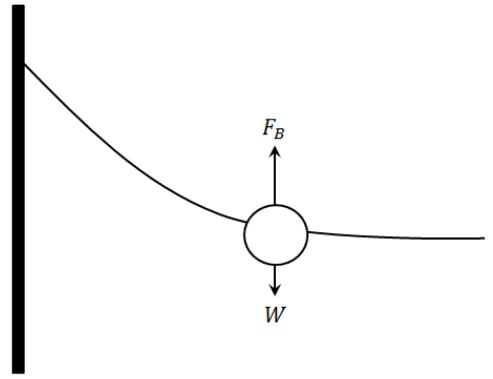
FIG. 3: The buoyant force,  $F_b$ , is greater than the weight,  $W$ , of the particle. This allows the particle to sit on the surface of the liquid. The particle can sit higher on the liquid surface if it moves left, up the meniscus, appearing to be attracted to the wall of the bowl.
