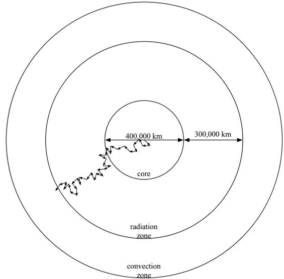
FIG. 2: (b) An illustration of a random walk of radiation from the core through the radiation zone of the Sun. As shown, scattering can cause a change in direction by a small amount or by an angle close to  $\pi$ . This is a simplified version, as the random walk can also cause the radiation to double back on itself, crossing through where it has already been.
