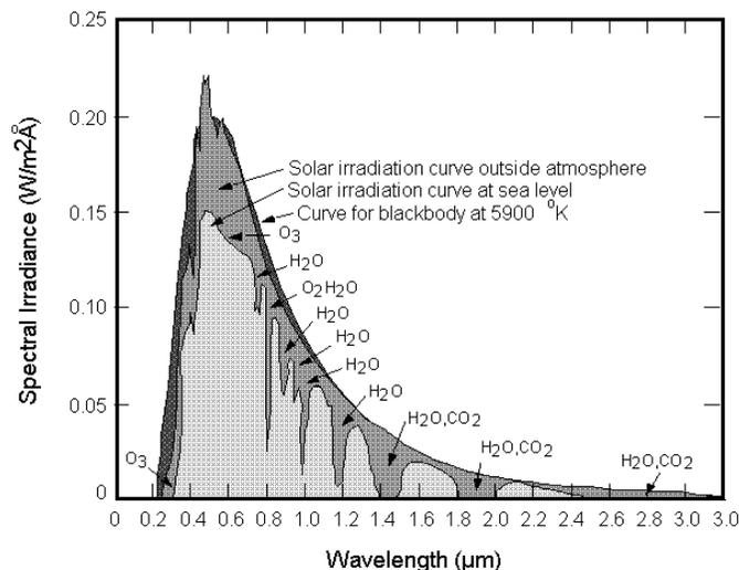
FIG. 1: The spectrum of the Sun as compared with a perfect blackbody spectrum. Figure courtesy of [5].
