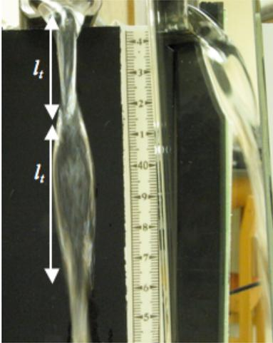
FIG. 4 – The frontal view is on the left and the side view is on the right. Notice that as the stream widens in one plane it contracts in the other.
