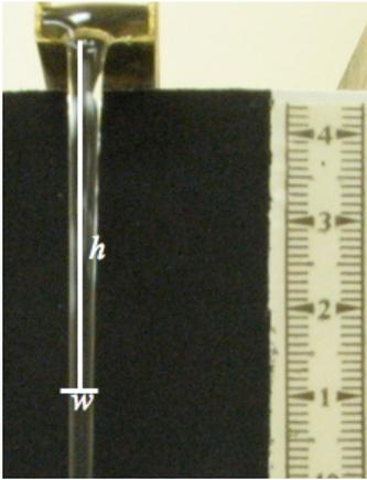
FIG. 2 – Example of a picture used to measure the contraction of a falling stream of water.
