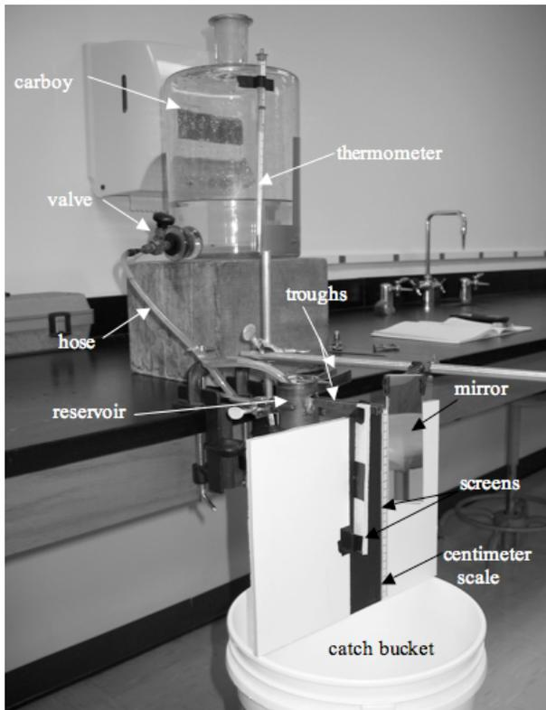
FIG. 1 – The setup used in the experiment.
