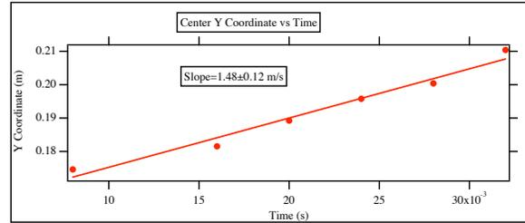
**Figure 1.5:** Graph of the Y-coordinate of center of mass versus time.
