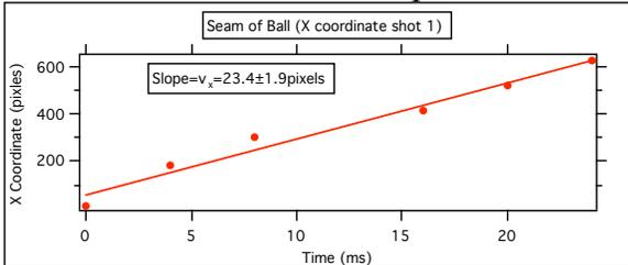
**Figure 1.2:** A graph of the path of the seam of the ball in the X-direction relative to the center of mass.
