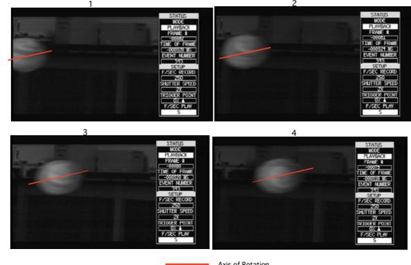
**Figure 1.1:** Consecutive frames over a time of 12 ms. Notice how the seam rotates about the line representing the axis of rotation.
