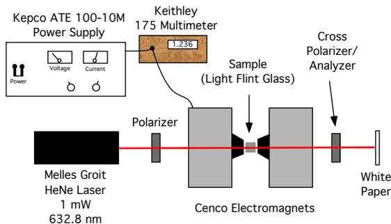
FIG. 1: A schematic of the setup used to measure the Verdet Constant.
