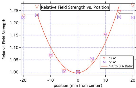
FIG. 3: A plot of the relative field strength  $B(x)/B(0)$  vs. position between the poles used to find an average value of the magnetic field experienced by the sample.
