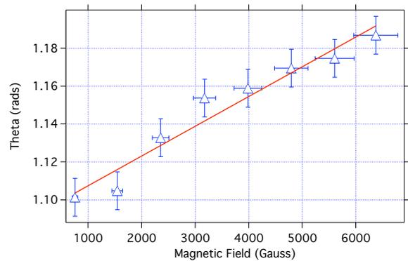
FIG. 4: A plot of the angle of rotation of the plane of polarization vs. the magnetic field with an associated linear fit.
