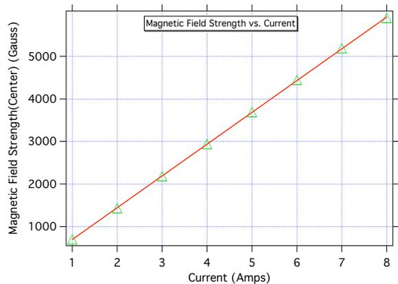
FIG. 2: A plot of the field strength vs. the current.
