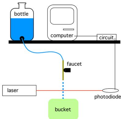
FIG. 3: A glass bottle was used as a reservoir for the water. This bottle was connected to the Nupro faucet, which could be finely adjusted to control the flow rate. The water dripped into a bucket set on the floor. To record the times of the drops, a laser was shone through the path of the drops, and its signal was recorded by a photodiode connected through a circuit to a computer.
