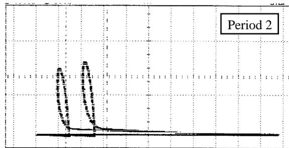
Figure 2. Phase space diagram of  $V_0$  versus  $V_S$  at Frequency = 180.0 KHz and Amplitude = 2.985 V<sub>pp</sub>. Period 2 is seen here as two peaks.
