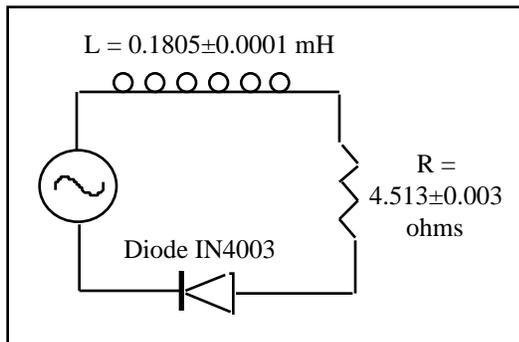
Figure. 1. Circuit diagram of setup for a driven nonlinear electrical oscillator. A function generator creates a current that travels through a conductor, resistor, and a diode.
