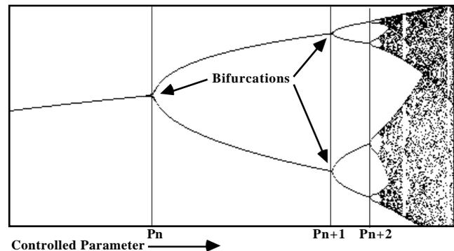
Figure 1 : An example of a numerically calculated bifurcation diagram exhibiting period doubling as the variable on the horizontal axis is varied.
