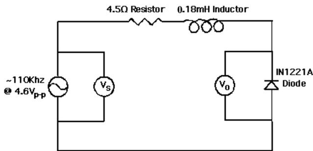
Figure 2 : Diagram of the chaotic circuit where  $V_S$  is the applied input voltage and  $V_O$  is the output voltage.
