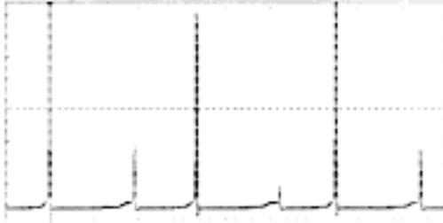
Figure 3 : An output signal time series with four distinct peaks showing a period four times that of the applied signal.
