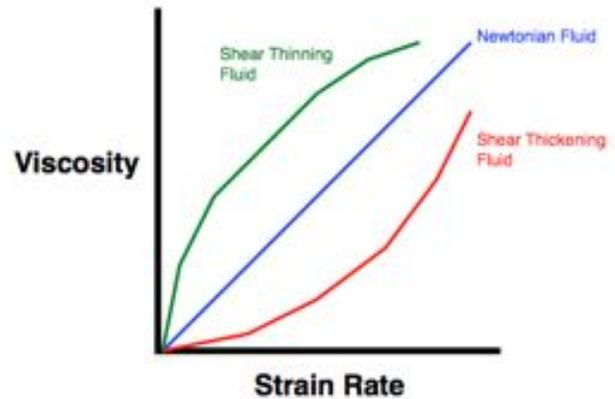
FIG. 1: A graph of how both Newtonian and Non-Newtonian fluids react under stress.
