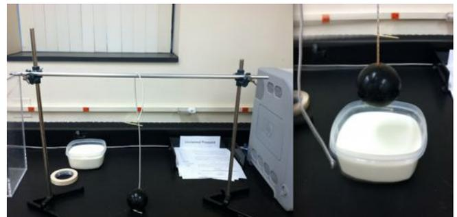
FIG. 3: My apparatus. On the left is the setup I used to suspend the ball, and on the right is an image of the ball suspended over the solution.
