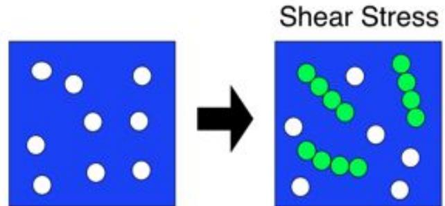
FIG. 2: A drawing of how the molecules shift when the STF experiences hydroclustering [2].
