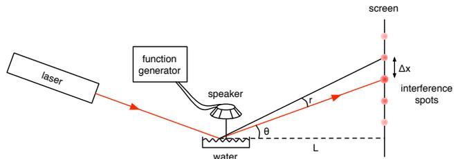
FIG. 1: A laser beam is aimed at a reservoir containing water, with ripples induced by a wire attached to a speaker driven by a function generator. The surface ripples act as a diffraction grating causing the interference spots on the screen.
