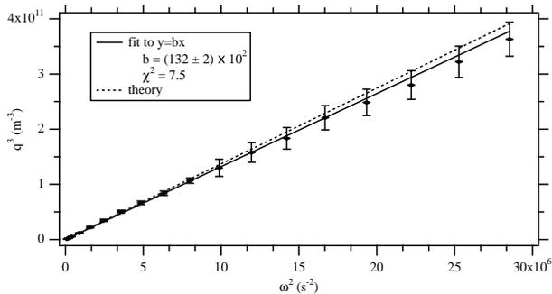
FIG. 6: Plot of  $q^3$  versus  $\omega^2$  fit to a line (solid) along with a line (dashed) corresponding to the expected slope of  $\rho/\sigma$ .
