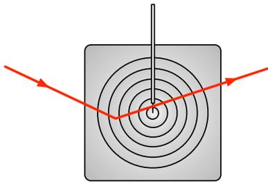
FIG. 2: The optimal spot to aim the laser is slightly off center and away from the wire.
