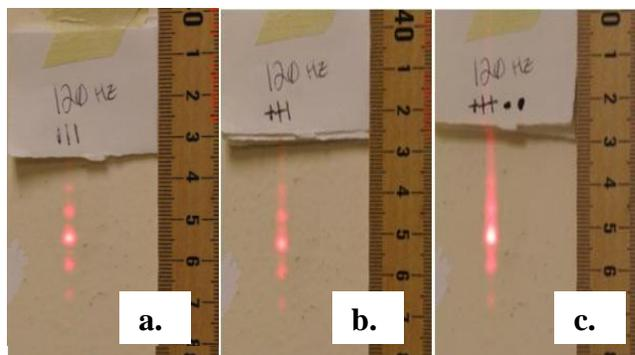
**Figure 5.** The reflection and interference spots at 120 Hz from chlorine water for a.) 0.5 ppm, b.) 2.0 ppm, c.) 3.0 ppm.
