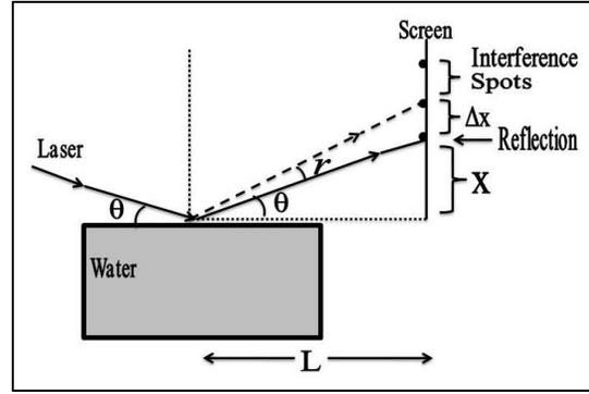
**Figure 2.** Diagram of the experiment with specific attention to the necessary measurements.
