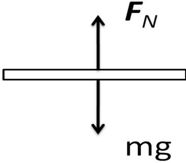
**Figure 1.** This is the free-body diagram of the plate, with  $F_N$  as the normal force from the water, and  $mg$  is the force due to gravity
