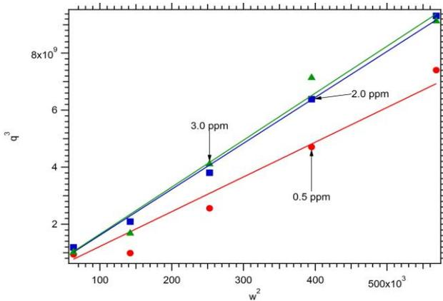
**Figure 8.** The slope of each of these linear fit lines is  $b$ , which I used to determine each water sample’s surface tension.
