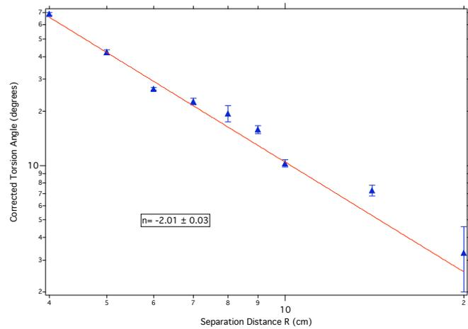
**Fig. 3** – This is the  $\log \theta_{\text{corrected}}$  vs  $\log R$  plot after the correction factor was applied to  $\theta$ . This line is also weighted heavier towards data points with less error.
