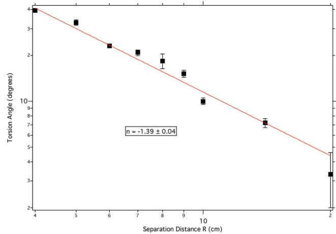
**Fig. 2** – This is the  $\log \theta$  vs  $\log R$  plot before the use of the correction factor on  $\theta$ . The line is weighted heavier to the data points with less error.
