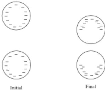
**Fig. 1** – In this diagram, the initial state represents the two spheres when they are far apart and act, to some degree, as point charges. The final state shows the two spheres close enough where the surface charges repel each other and repel to opposite ends of the spheres.
