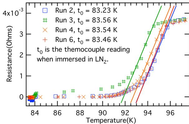
FIG. 5: Plot of resistance versus temperature of the superconductor for runs 2, 3, 4, and 6.
