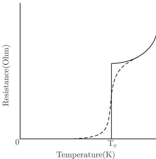
FIG. 2: The solid line shows the resistance versus temperature for a perfect superconductor crystal while the dotted line shows the expected curve of an imperfect superconductor. Based off of a figure from reference [4].
