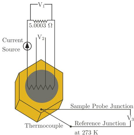
FIG. 4: Diagram of the four-point probe and thermocouple of the superconducting sample.
