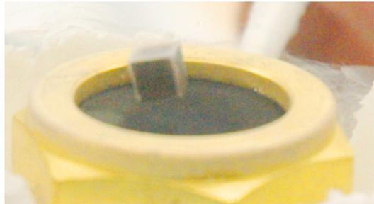
FIG. 1: A neodymium magnet levitating above a YBCO type superconductor.
