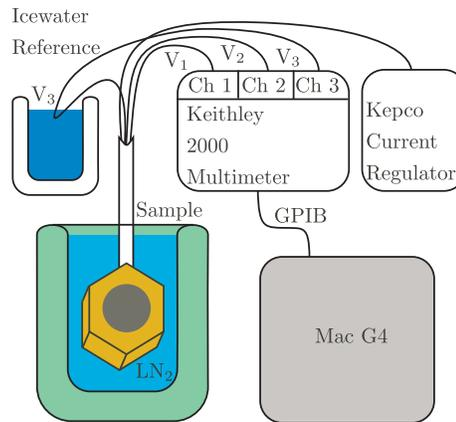
FIG. 3: Schematic of the experiment set up with the sample suspended in the liquid nitrogen bath. Diagram after reference [6].
