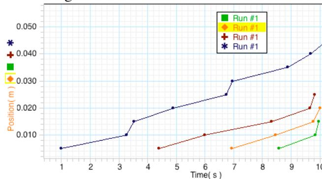
Figure 4: An example of the data obtained from Data Studio, using photogates to monitor the movement of each block, with each line representing a different block.
