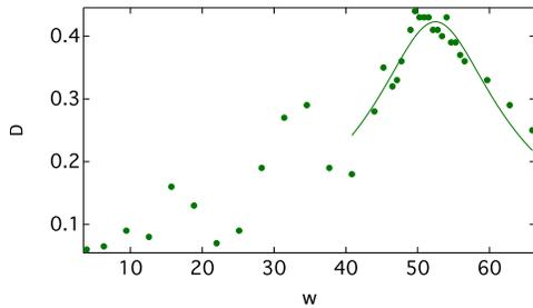
FIG. 4: Amplitude of Oscillation (meters) vs  $\omega$  (Hz). Q value is  $\omega_0/\text{FWHM}$  where  $\omega_0$  is the resonance frequency. This is for the bridge deck made of balsa wood.
