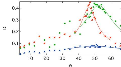
FIG. 7: Amplitude of Oscillation (meters) vs  $\omega$  (Hz). Q value is  $\omega_0/\text{FWHM}$  where  $\omega_0$  is the resonance frequency. The colors and shapes are the same as before with the other graphs.
