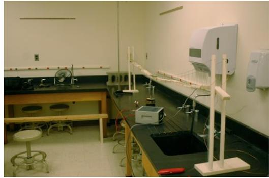
FIG. 2: Bridge set up with the birch wood deck. The plastic pipe supports and copper wire can be seen.
