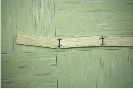
FIG. 1: Balsa wood deck with the eight holes drilled in it. Four for attaching the deck to the copper wire and four for attaching the section to other sections.
