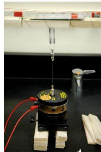
FIG. 3: PASCO driver attached to the side of the bridge deck.
