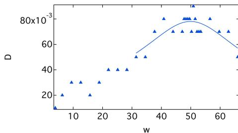
FIG. 5: Amplitude of Oscillation (meters) vs  $\omega$  (Hz). Q value is  $\omega_0/\text{FWHM}$  where  $\omega_0$  is the resonance frequency. This is for the bridge deck made of birch wood.
