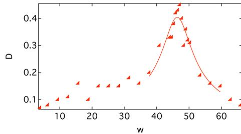
FIG. 6: Amplitude of Oscillation (meters) vs  $\omega$  (Hz). Q value is  $\omega_0/\text{FWHM}$  where  $\omega_0$  is the resonance frequency. This is for the bridge deck made of balsa wood with holes drilled into it.
