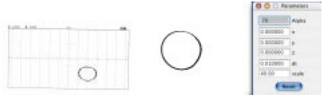
**Figure 1: Oscilloscope printout of period-1, A = 0.578, R = 1.73 K $\Omega$ . The screenshot on the left is of the numerical simulation showing period 1. Note that A, which in the dialog box is labeled as alpha, is equal to 0.78.**
