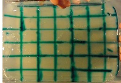
FIG. 1: Photo showing the gelatin slab with the grid marker and no wave propagating through.
