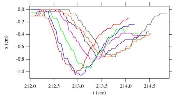
FIG. 2: Graph showing the movement of each vertical line in mixture 1 gelatin as the wave propagated through.
