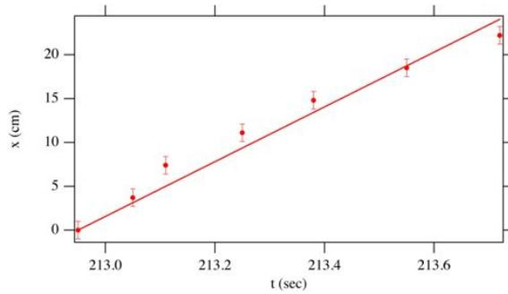
FIG. 3: Graph showing distance versus time of the wave propagating through mixture 1 gelatin with the slope of the fit line being the speed of the wave.
