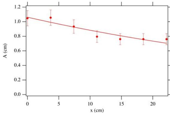
FIG. 4: Graph showing amplitude of the wave versus time at one time, with an exponential fit line representing the damping, in mixture 1 gelatin.
