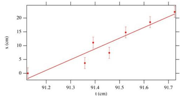
FIG. 6: Graph showing distance versus time of the wave propagating through mixture 2 gelatin with the slope of the fit line being the speed of the wave.
