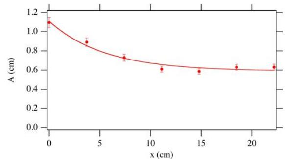
FIG. 7: Graph showing amplitude of the wave versus time at one time, with an exponential fit line representing the damping, in mixture 2 gelatin.
