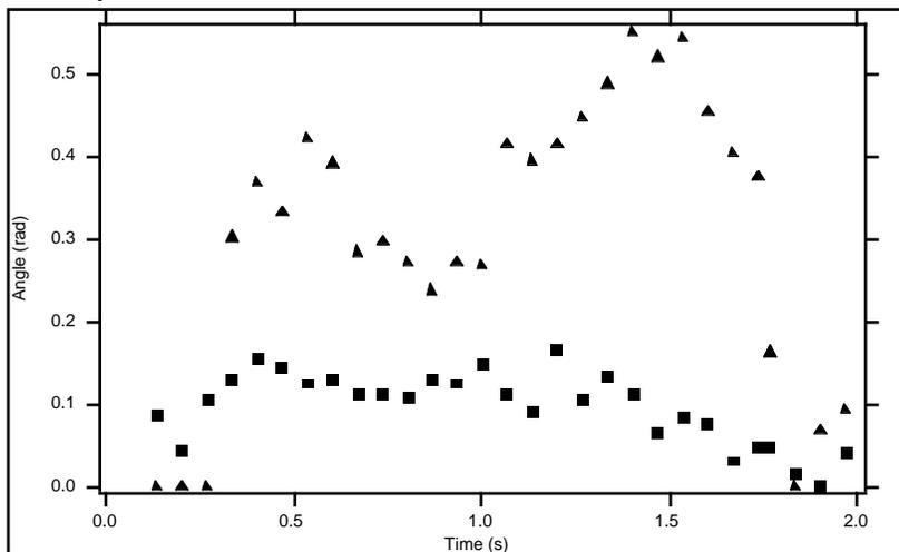
Fig 3. Steering angle (triangular markers) and Lean angle (square) with respect to time. The time units are in seconds, but are arbitrary
