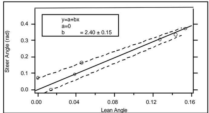
Fig 4. Steer angle versus lean angle. The plot displays a relationship between Steer angle and lean angle. Dotted lines represent bounds of region in which the actual line should
