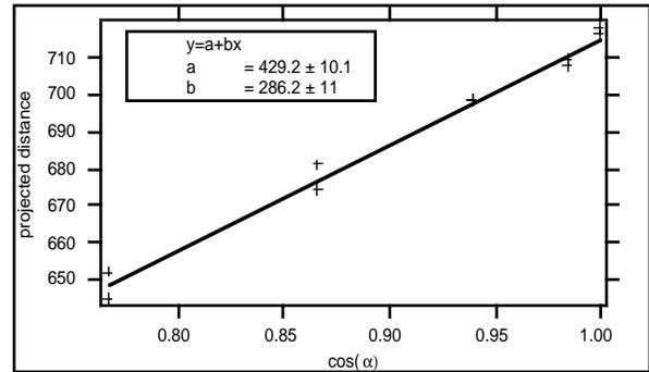
Fig 2. Projected distance between brake levers vs.  $\cos(\alpha)$ . Distance is in pixels.
