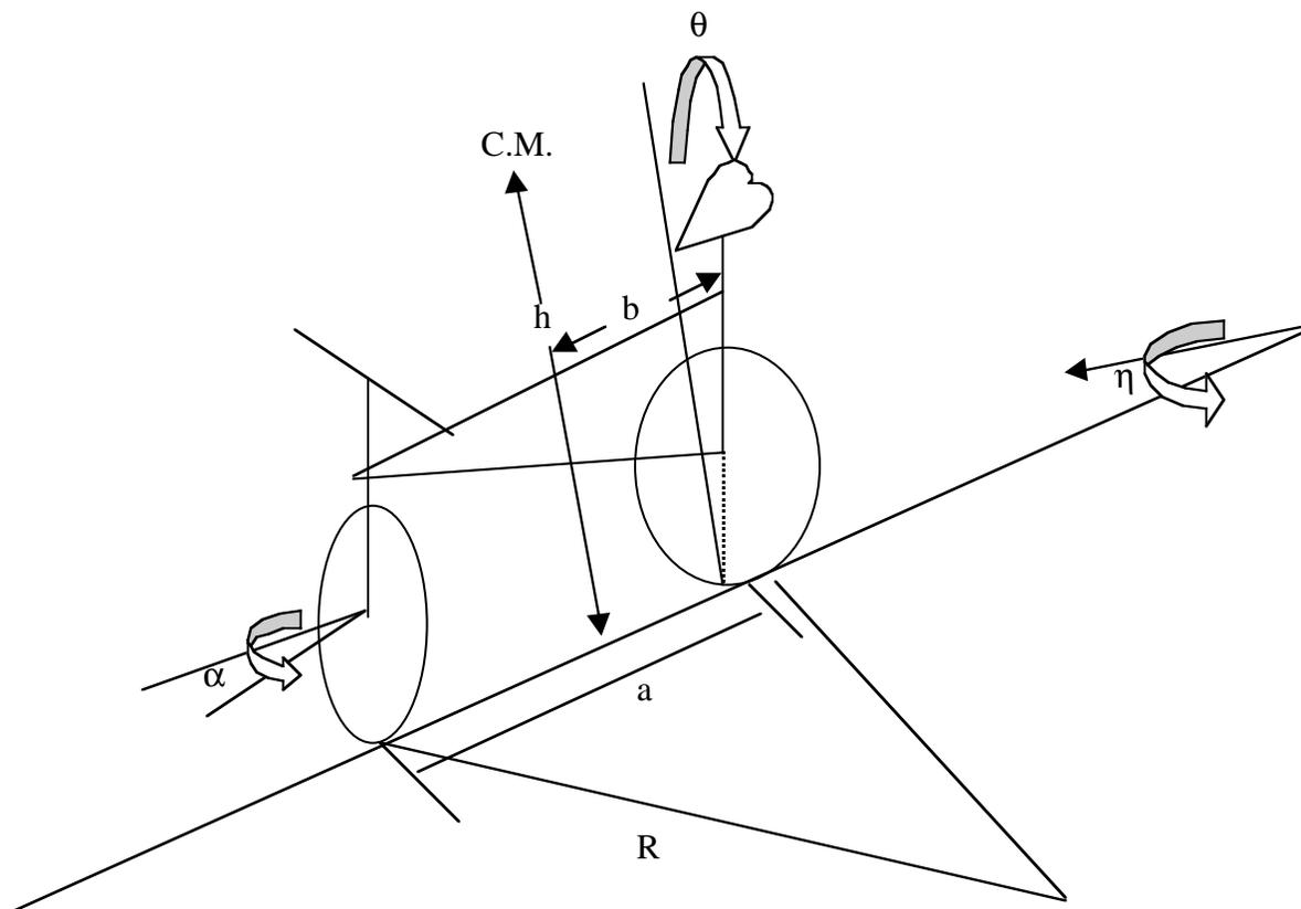
Fig 1. (From source 1) Bicycle and pertinent variables and parameters.  $\eta$  is the angle that a line connecting the contact points of the two wheels makes with some arbitrary horizontal reference vector.
